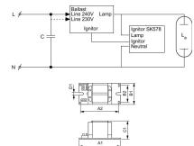
Scheda tecnica Lampada HID Philips BSN 400 K407-ITS 230/240V 50Hz
